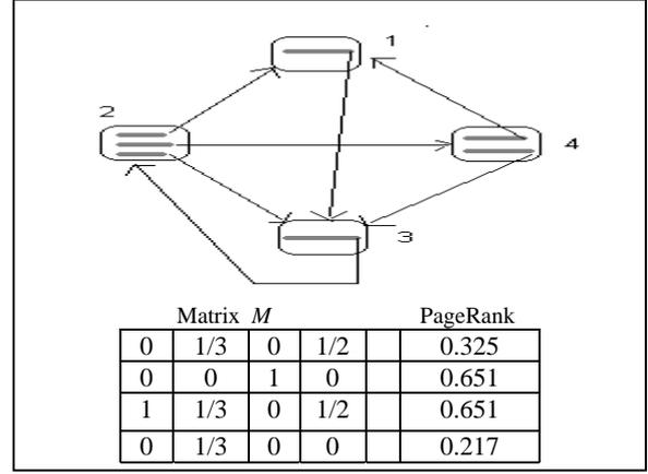
Figure 2. A small Web, its graph  $G$ , matrix  $M$ , and PageRank values (eigenvector corresponding to eigenvalue 1).
